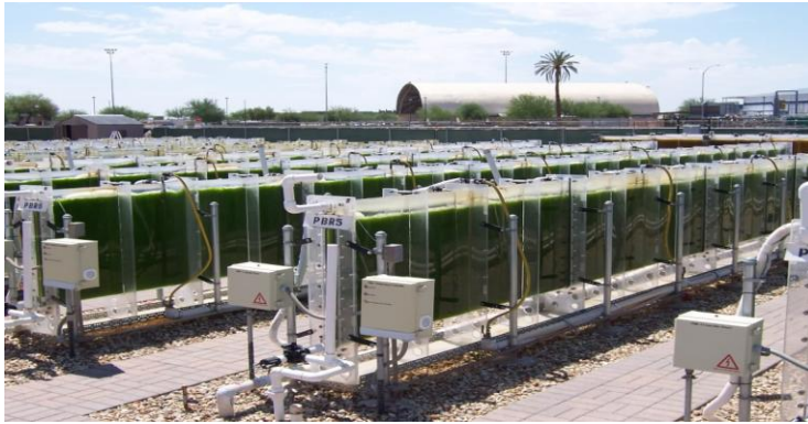
Figure 7; A flat plate photobioreactor system
